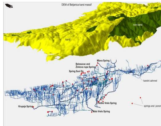
Fig. 3 3-D network of Beljanica aquifer karst channels
